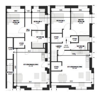
Figure 15 Floor plan of Maisonette Type 7.5 (left) and floor plan of Maisonette Type 7.6 (right).
